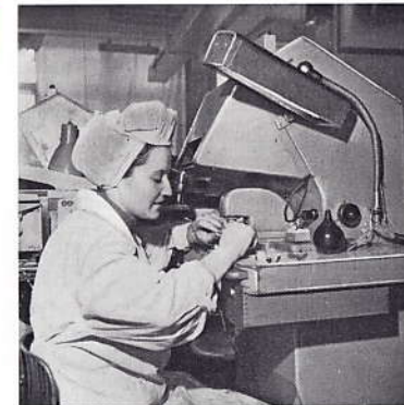
Up-to-date projector helps the girl at the most responsible point of watch assembling
