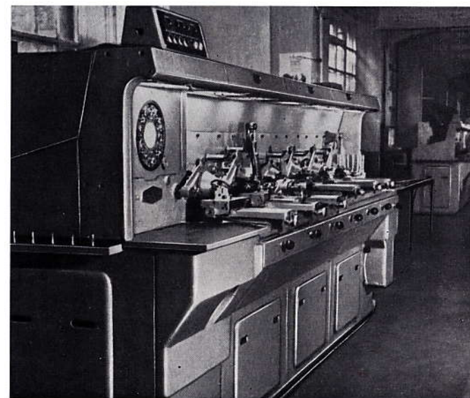
Automatic line installed at the 1st Moscow Horological Factory for machining watch cases
